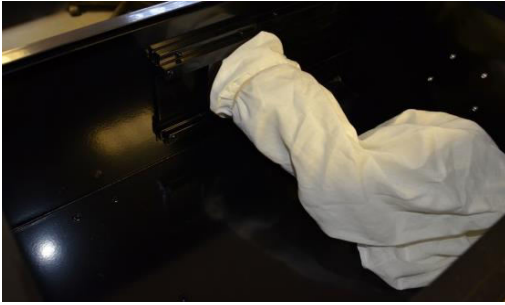
Figure 6: showing a modification of the trap box, to aid bagging snakes for transport. A cotton bag / pillow case is secured to the tube attachment so when the slide is open the animal enters the hole and directly in to the bag. Then by using remote handling tools the bag is removed from the tube and tied, containing and securing the animal in the bag ready for transport.
