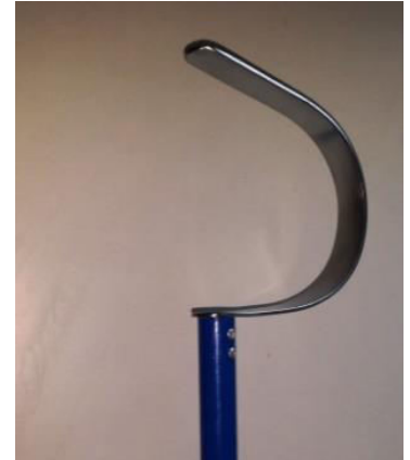
Figure 16: showing a modified hook plate with a larger surface area to distribute weight of a heavy bodied snake when handled.
