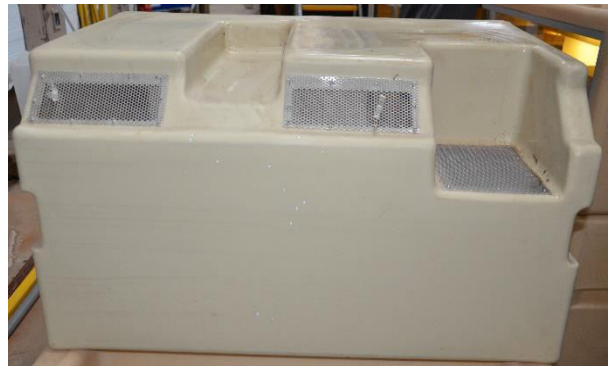
Figure 10: showing the back of a mould formed fibre glass vivarium where heating and lighting can be installed externally.
